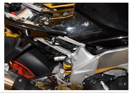
Plug the CESE connectors to the suspension connectors.
