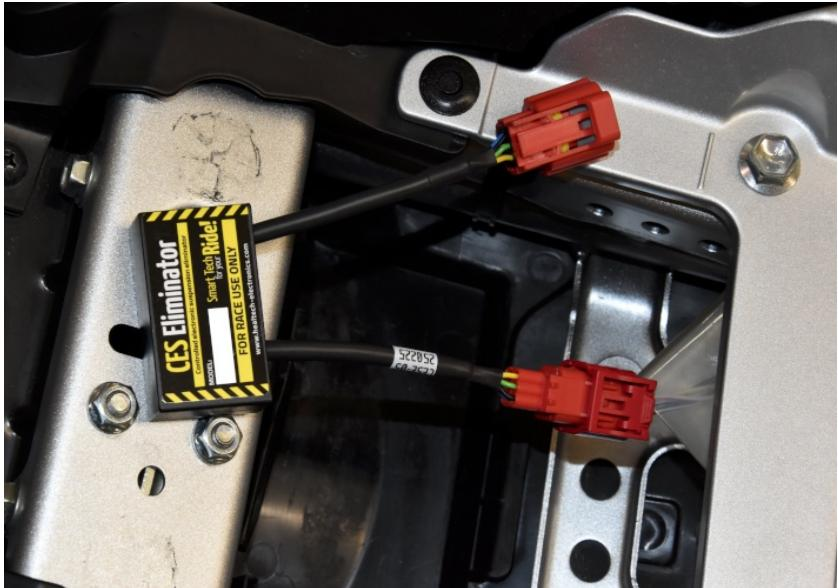
Typical position for the Controlled Electronic Suspension Eliminator.
