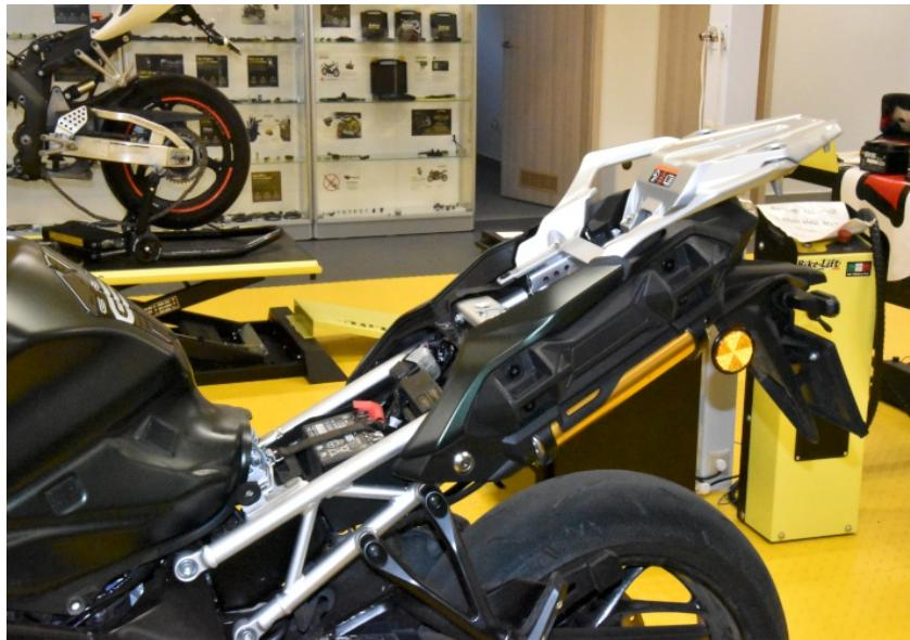
Locate the and remove the Suspension Control Unit.
