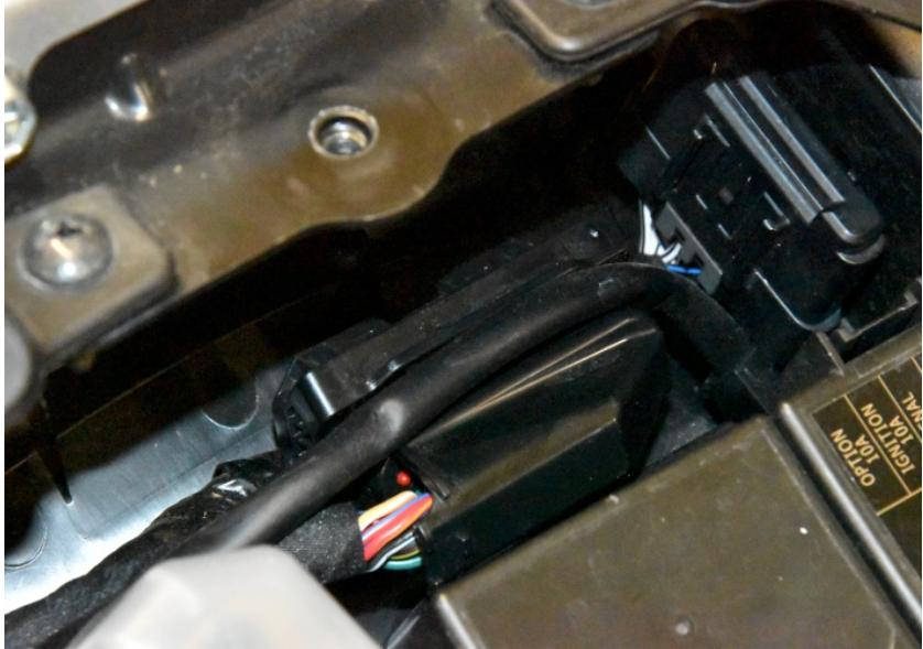
Plug the CESE connector to the diagnostic connector.
