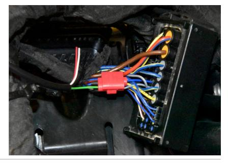
Splice the CESE White wire to the Grey wire of the SCU connector. Use a red wire tap connector.
