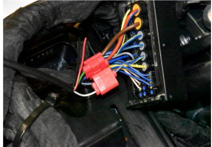
Splice the CESE Black wire to the Brown wire of the SCU connector. Use a red wire tap connector.
