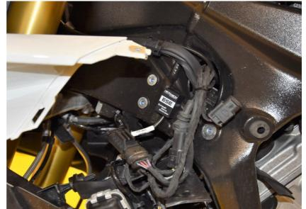
Locate the 2nd Exhaust Servo motor.
