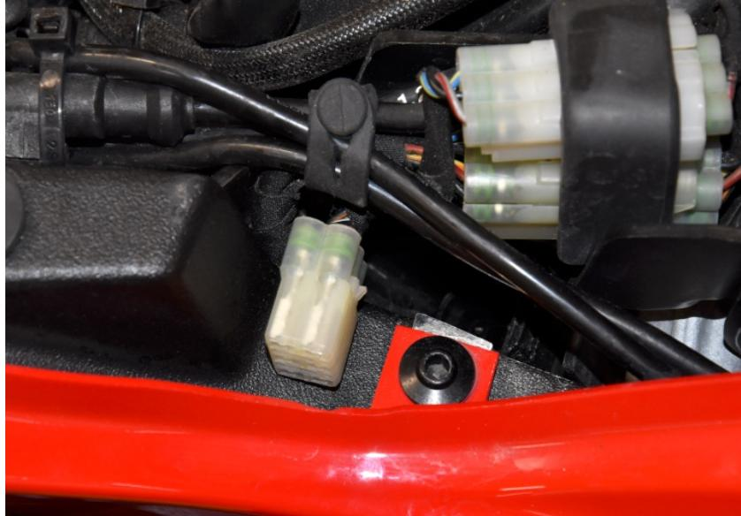
Plug the ESE connectors to the exhaust servo motor connectors.
