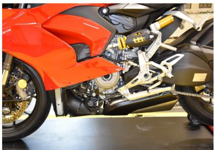
Locate the Exhaust Servo-motor and it's black, 6-pole connector.
