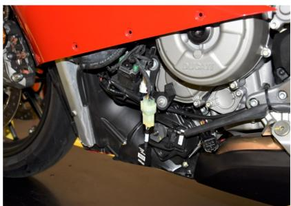
Typical position for the Exhaust Servo Eliminator.
