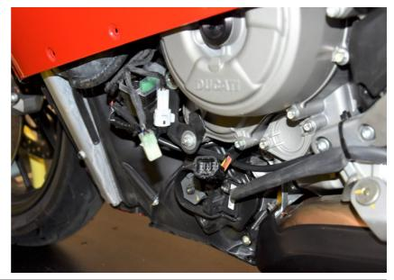
Plug the ESE connector to the Exhaust Servo-motor connector.
