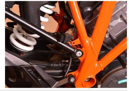
Install the KTM retaining bracket (#61613968044) for the rear brake reservoir.
