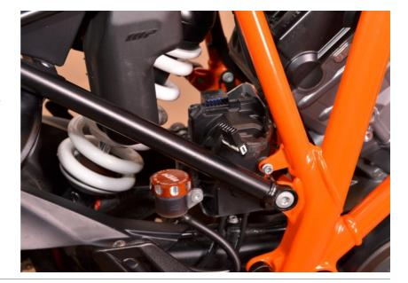
Remove the exhaust servo motor completely with the middle pipe and install an aftermarket middle pipe or full exhaust.
