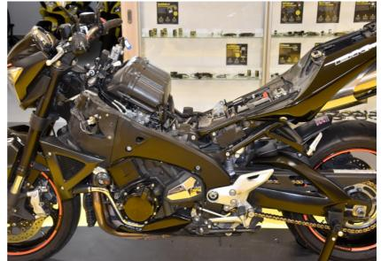
Locate the Exhaust Servo-motor under the fuel tank.
