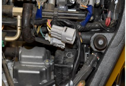
Remove the exhaust servo motor.
