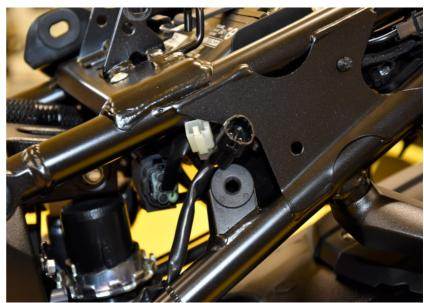
Remove the exhaust servo motor.
