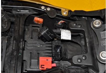
Plug the FI Cleaner Tool connector to the diagnostic connector.
