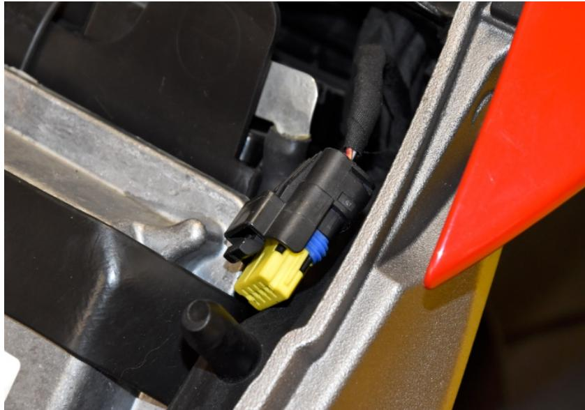
Plug the FI Cleaner Tool connector to the the diagnostic connector.
