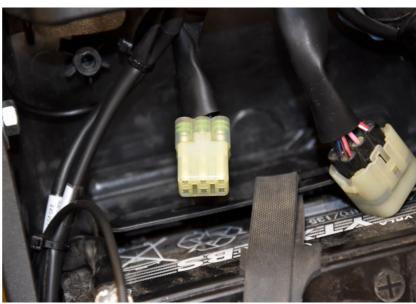
Plug the FI Cleaner Tool connector to the the diagnostic connector.
