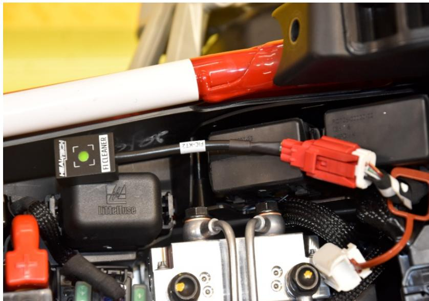
Turn the ignition key ON. The LED shows the current status of the maintenance.
