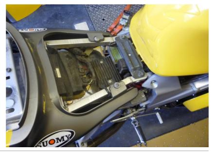
Plug the FI Tuner Pro connector to the Expansion Port.
