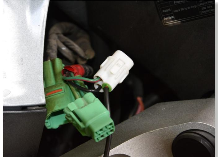
RELEASE AND REMOVE THE GREEN/RED AND BLACK/YELLOW WIRES FROM MALE CONNECTOR.
