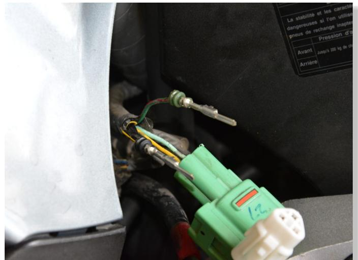
INSERT THE TWO MALE METAL CONTACTS INTO THE LARGER 3-POLE TRIANGULAR PLUG THROUGH THE BACK UNTIL THEY CLICK INTO PLACE.
