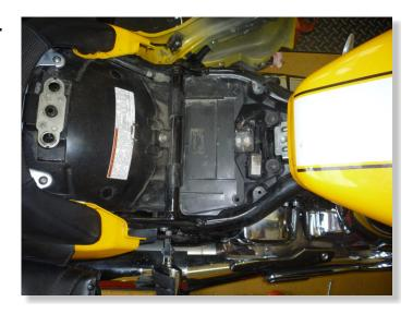
REMOVE THE LEFT AND RIGHT FRAME COVERS BELOW THE SEAT AND FUEL TANK.
