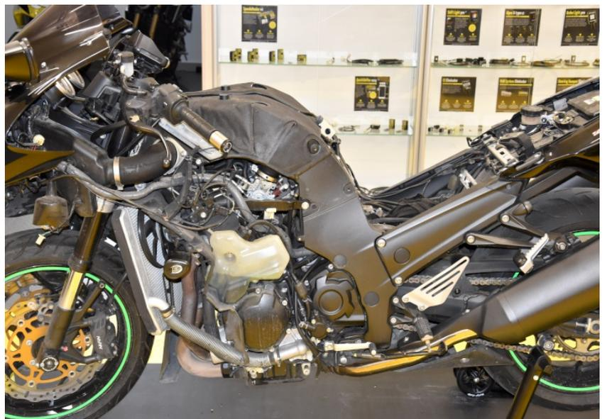
Locate the green, 4-pole gear position sensor connector under the airbox and disconnect it.
