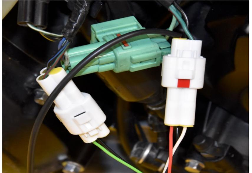
Connect the GPAT G2 Red wire to the Blue wire of the brake light switch 2-pole connector.
