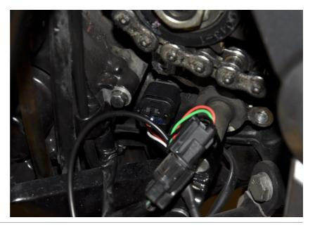
Connect the GPAT Red wire to the White/Red wire of the fuel pump connector.
