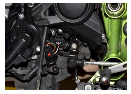
Connect GPAT G2 Red wire to the Brown/Yellow wire of the ABS indicator light at the 2-pole connector.
