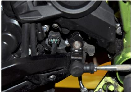
Remove the chain cover and route the GPAT G2 harness to the plug.
