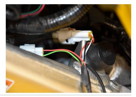
Connect the GPAT Red wire to the Yellow/Red wire of the fuel pump connector.
