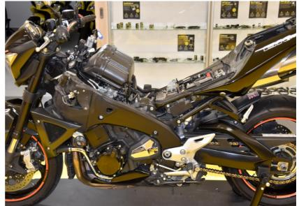
Locate the white, 3-pole gear position sensor connector under the fuel tank.
