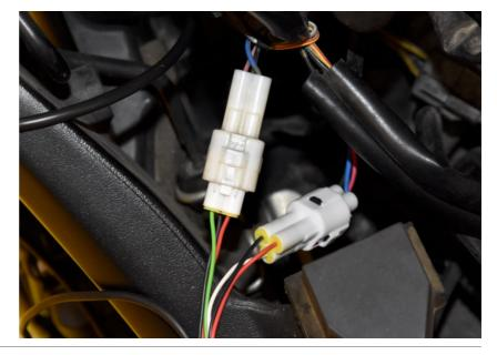
Connect the GPAT Red wire to the Orange wire of the rear brake light switch connector.
