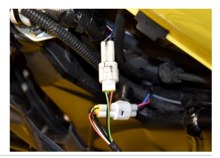
Connect the GPAT G2 Red wire to the Yellow/Red wire of the fuel pump relay connector.
