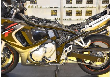
Locate the white, 3-pole gear position sensor connector under the seat.
