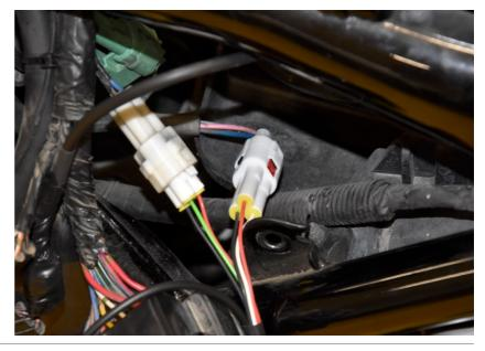
Connect the GPAT Red wire to the Orange/Green wire of the diagnostic connector.
