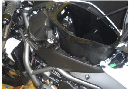
Remove the battery plastic cover inside helmet holder box.
