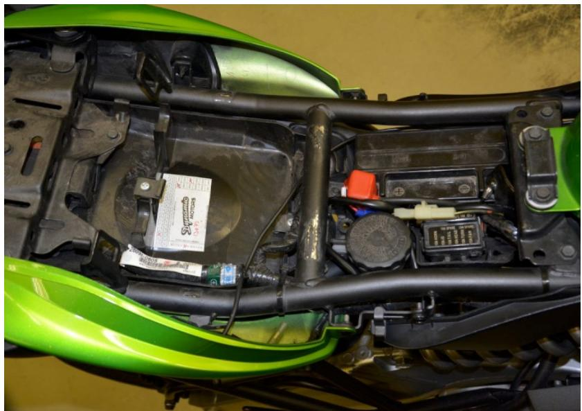
Connect the Gipro connector to the diagnostic system connector.
