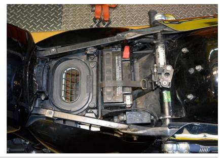
Remove the intake/side cover from left side.
