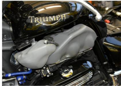
Lift up or remove the fuel tank.
