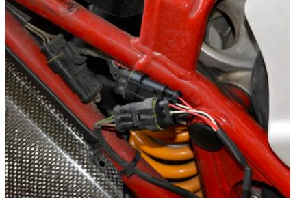
Connect the GPX Black/Green wire to the Brown wire of the crankshaft position sensor connector.
