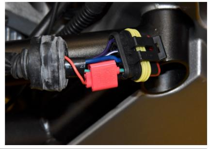
Connect the GPX Black/Green wire to the White wire of the crankshaft position sensor connector.
