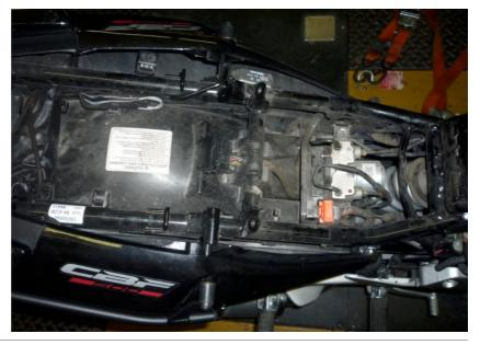
Remove the Black frame covers at both side from under the fuel tank.
