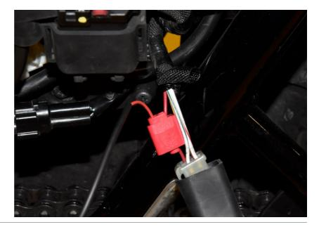
Connect the GPX Black/Green wire to the Yellow wire of the crankshaft position sensor connector.
