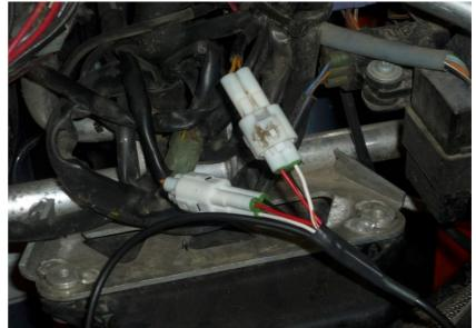
Connect the GPX Black/Green wire to the White/Blue wire of the tacho dashboard connector.
