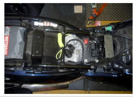
Lift up or remove the fuel tank.
