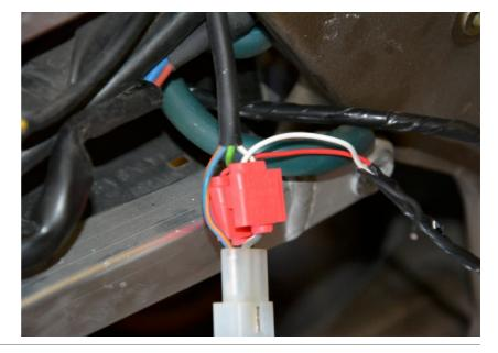
Connect the GPX Black wire to the Blue/Orange wire of the speed sensor connector.
