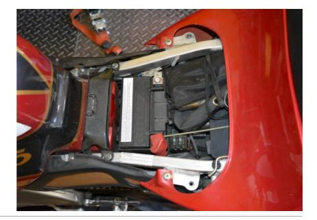
Locate the speed sensor connector on the right side under the frame cover.
