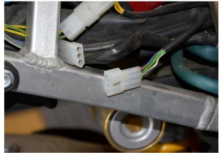
Connect the GPX Red wire to the Green wire of the speed sensor connector.
