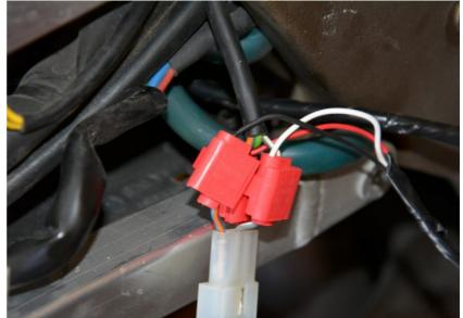
Connect the GPX Green wire to the Orange/White wire of the ignition coil under the middle fairing on the right side.
