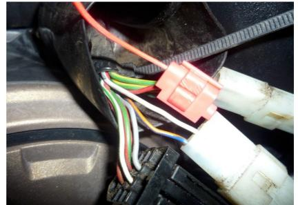
Connect the GPX White wire to the Gray/White wire of the speed sensor connector.
