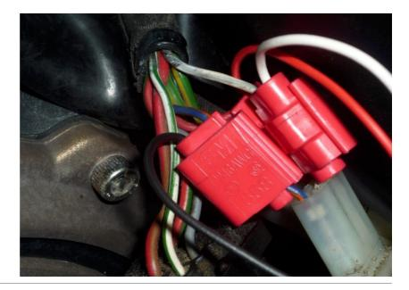
Connect the GPX Green wire to the Blue/Yellow wire of the Camshaft Position Sensor connector.
