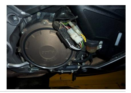
Connect the GPX Red wire to the Red wire of the speed sensor connector.
