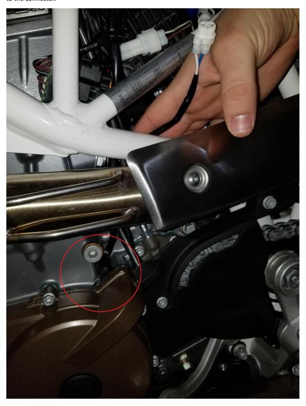
Note: the HealTech Universal wire harness may need some modification depending on motorcycle model. In this case the green wire from the HealTech harness must be run through the motorcycle to the Crankshaft Position Sensor while the Red, White, and Black wires from the HealTech harness need to be routed to the headlight assembly.
