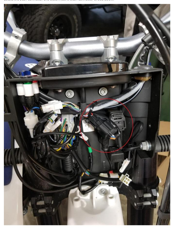
Shown below is the side of the connector we will splice the Red, Black, and White wires into from the GPX harness .
