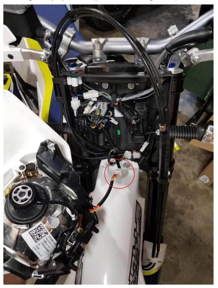
Locate the Dash Connector and disconnect it. Dash Connector circled below.
