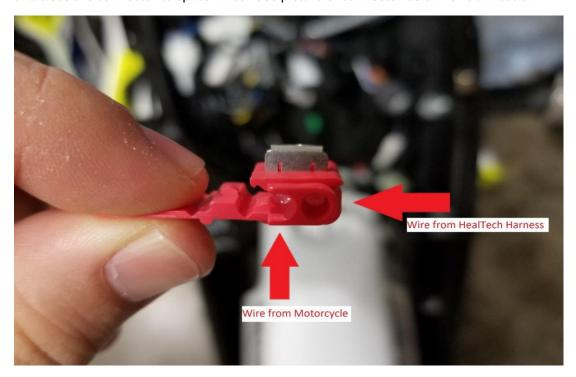
Below you can see how the connector should look prior to closing the connector.
