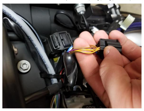
On the left side of the motorcycle locate the Crankshaft Position Sensor circled below. The Crankshaft Position Sensor is a 2-pole connector with a White/Yellow and Yellow/Blue wire. Specific location of this connector may very by bike based on other aftermarket parts being installed.
