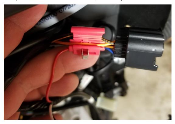
After connecting all three wires from the Dash Connector plug, plug in the HealTech gear indicator to the harness and turn the motorcycle key to the "ON" position while in Neutral gear. The indicator should count down from 7 then blink L slowly. This indicates you have correctly connected the Power (Red), Ground (Black) and the Speed Sensor (White). See pictures below for correct connector appearance and Dash/Gear Indicator display.
