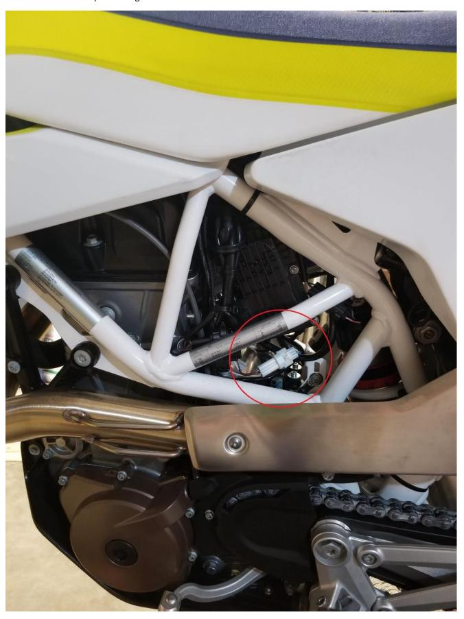
The Crankshaft Position Sensor can be identified by tracing the connector from the top of the Crankcase (circled below) to the connector.
