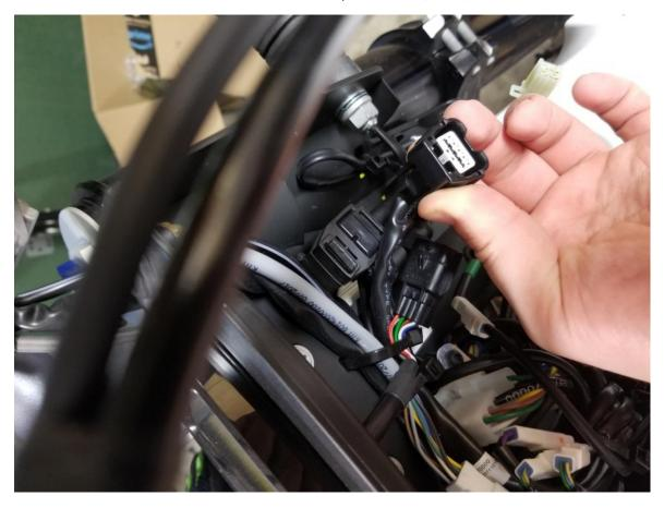
Peel back the sleeve on the connector and separate the Black/Orange, Orange, and Brown/Violet wires.
