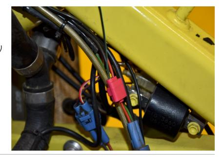
Connect the 3-pole sensor connector to the GPX wiring harness connector.
