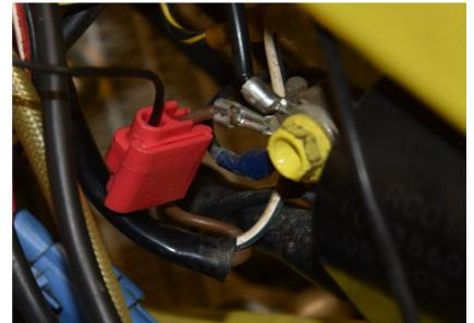
Connect the GPX red wire to the battery positive terminal via an on/off switch.
