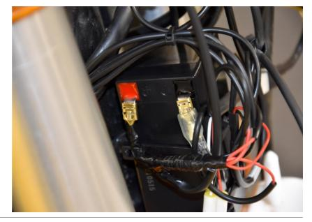
Connect the GPX Black/Green wire to the White/Blue wire of the ignition pulse generator connector.
