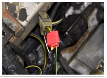
Connect the GPX Red wire to the Brown wire of the black multi connector under the fuel tank.
