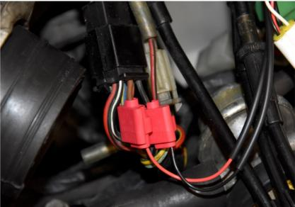
Connect the 3-pole wheel speed sensor connector to the GPX wiring harness connector.
