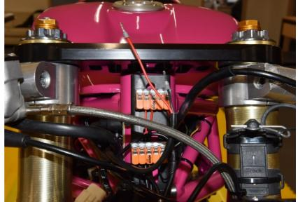
Connect the 3-pole sensor connector to the GPX wiring harness connector and coil up the excess length.
