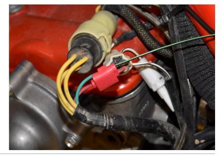
Connect the GPX Black wire to the Blue wire of the 8-pole transparent multi connector under the fuel tank.
