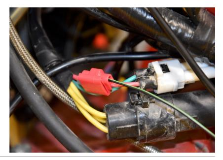
Connect the GPX Red wire to the Brown/White wire of the 4-pole black multi connector under the fuel tank.
