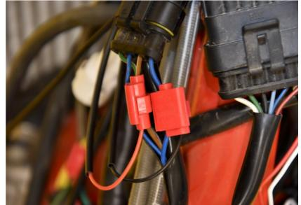
Connect the 3-pole wheel speed sensor connector to the GPX wiring harness connector.
