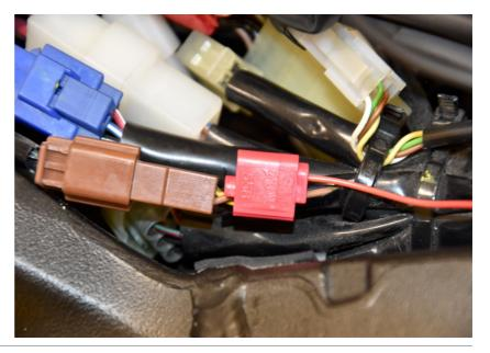
Connect the GPX Black/Green wire to the Gray wire of the crankshaft position sensor connector.
