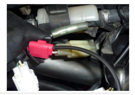
Connect the GPX Red wire to the Brown wire of the rear brakelight switch connector.
