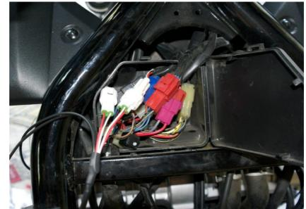
Connect the GPX Black/Green wire to the Gray wire of the crankshaft position sensor connector.
