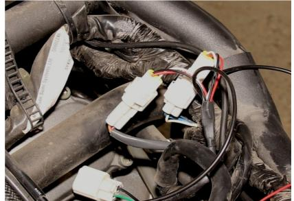
Connect the GPX Black/Green wire to the Gray wire of the ECU connector.
