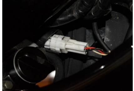
Connect the GPX Black/Green wire to the Blue wire of the Crankshaft Position Sensor connector.
