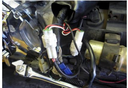
Connect the GPX Black/Green wire to the Orange wire of the ECU/ECM connector.
