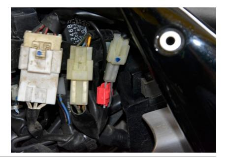
Connect the GPX Red wire to the Brown wire of the rear light connector.
