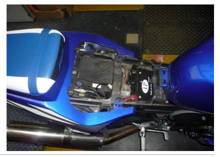
Lift up or remove the fuel tank.
